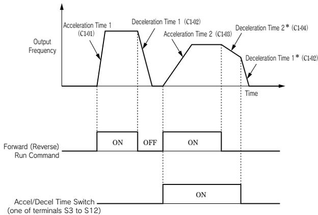
\* When stopping method is deceleration to stop (b1-03=0).
