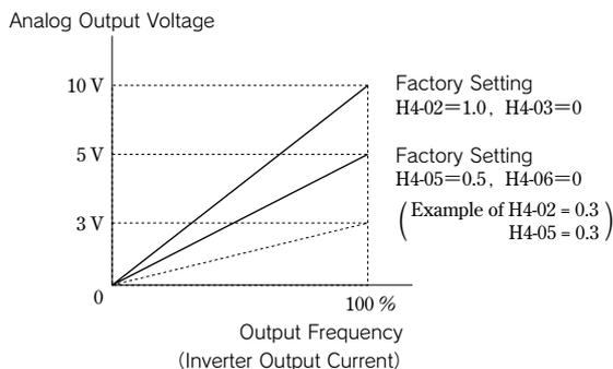
For frequency meter that displays 0 to 60 Hz at 0 to 3 V
