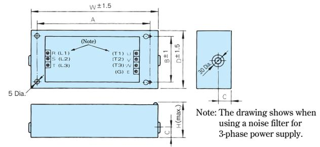
Note: The drawing shows when using a noise filter for 3-phase power supply.
