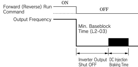
The DC injection braking time is as follows, according to the output frequency when stop command is input.
