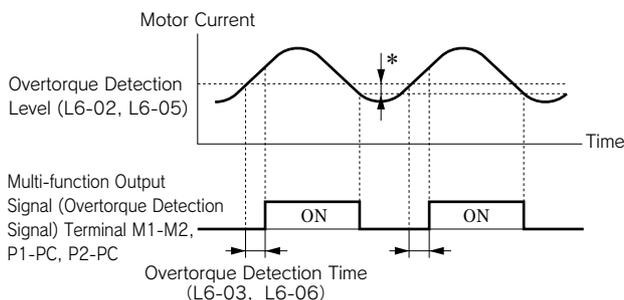
\* The releasing width of overtorque detection is approx. 10 % of the inverter rated current (or motor rated torque).
