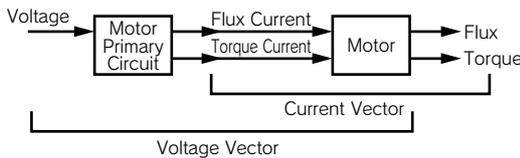
This control can be equivalent to the current vector if the primary circuit of the motor is known completely, but this is actually difficult since the temperature of the resistance also changes.
