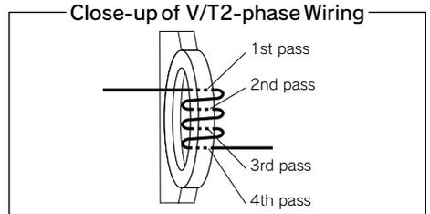
Pass each wire (U/T1, V/T2, W/T3) through the core 4 times.
