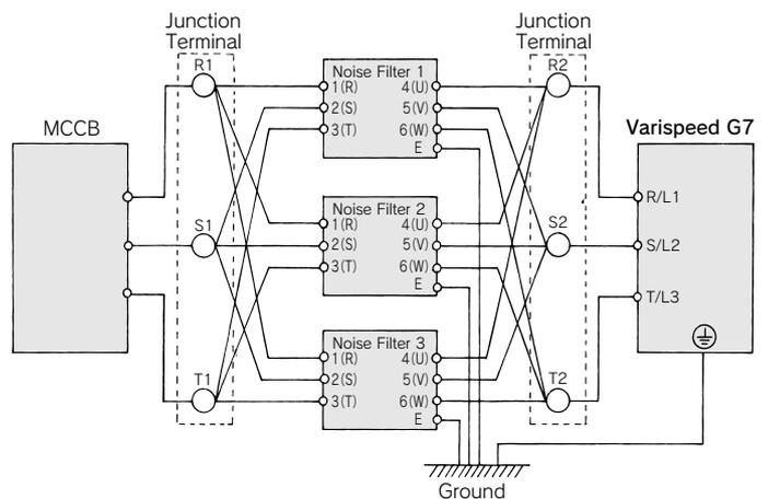
When wiring contactors in parallel, make sure wiring lengths are the same to keep current flow even to the relay terminals. Ground wires for noise filter and inverter should be thick and as short as possible.
