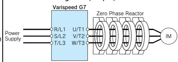
Put all wires (U/T1, V/T2, W/T3) through 4 cores in series without winding.
