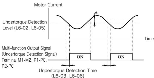
\* The releasing width of undertorque detection is approx. 10 % of the inverter rated current (or motor rated torque).
