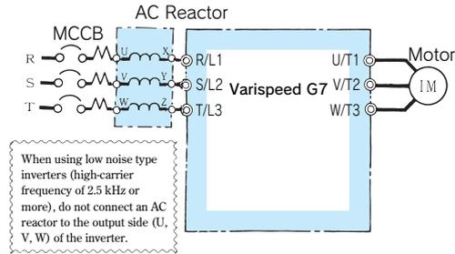
When power capacity is significantly greater when compared to inverter capacity, or when the power-factor needs to be improved, connect the AC or DC reactor.
