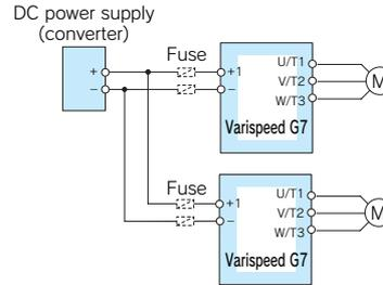
Note: When connecting multiple drives together, make sure that each drive has its own fuse. If any one fuse blows, all fuses should be replaced.
