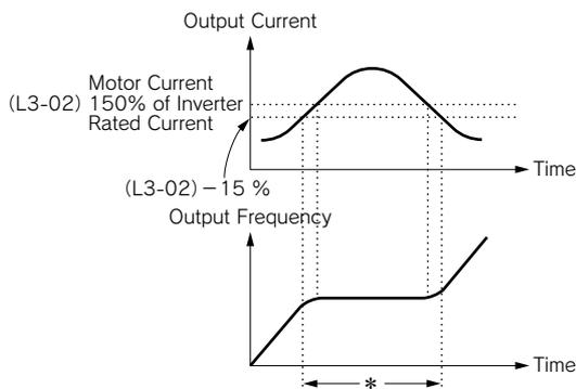
\* Output frequency is controlled so that stall status may not be caused in the meantime.
