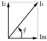
The primary current size  $I_1$  and phase  $\phi$  and controlled simultaneously.
