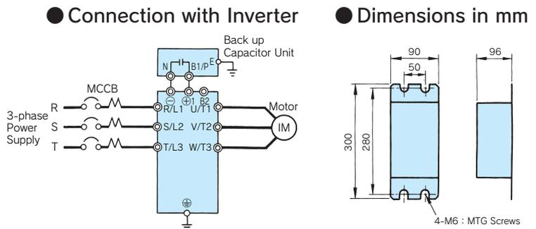
\* When this unit is not used, the inverter's power loss ride-thru ability is 0.1 to 1 second.
