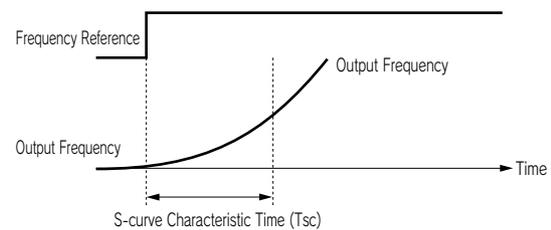
Setting the S-curve characteristic time, the acceleration or deceleration time will be longer by 1/2 of the S-curve characteristic time at start or end.
