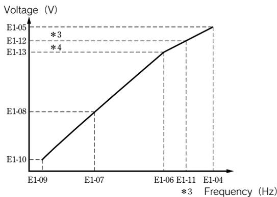
Set E1-04 to 11 so that  $E1-04 \geq E1-11 \geq E1-06 \geq E1-07 \geq E1-09$ . To make the line of the V/f characteristics straight, set E1-07 and E1-09 to the same value. At this time, the set value of E1-08 is disregarded. E1-11, 12 and 13 must be set only at V/f minute adjustment in the constant output area. Normally, they do not have to be set.
